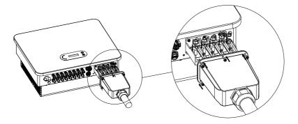
Figure 4-9 AC cable connection instruction diagram (2)
