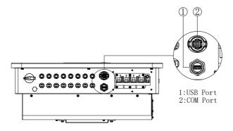
Figure 4-16 Communication connection Port
