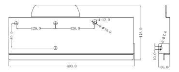
Figure 2-5 bracket dimensions (take 50KW for example)
