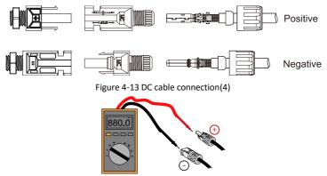
Figure 4-14 Use a multimeter to check the positive and negative electrodes
