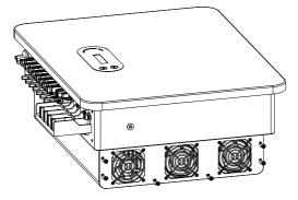
Step 2: Unscrew six screws at the corner of fans baseboard ;
