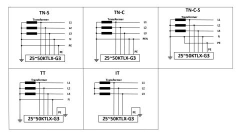
Figure 2-2 Overview of the grid configurations
