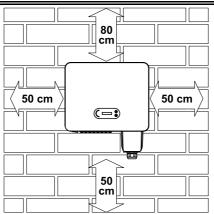
Figure 3-2 Clearance for single inverter
