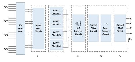
Figure 2-8 Schematic diagram(take 50KW for example)
