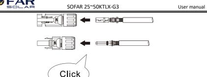
Figure 4-12 DC cable connection(3)
