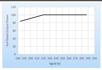
Figure 2-10 Rated Power ratio vs Grid Voltage
