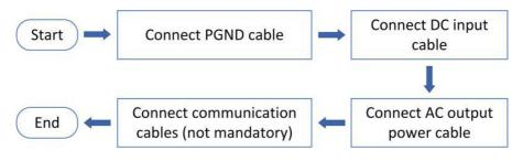
Figure 4-1 flowchart for connecting cables to the inverter
