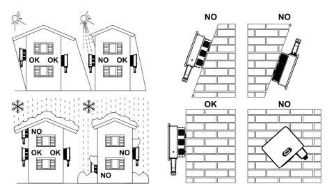
Figure 3-1 Installation Position Selection
