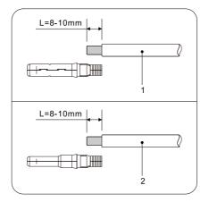
Figure 4-10 DC cable connection (1)
