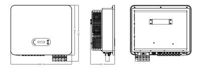
Figure 2-3 Front, side and back of the machine (take 50KW for example)
