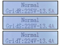
Inverter working status, grid voltage and frequency
