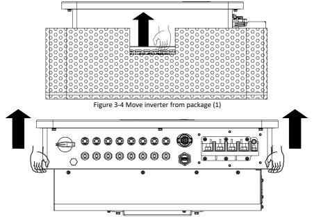
Figure 3-5 Move inverter from package (2)
