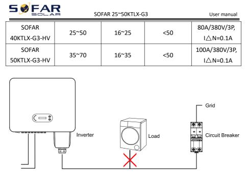
Figure 4-5 Incorrect connection between load and inverter
