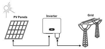
Figure 2-1 PV Grid-Tied System
