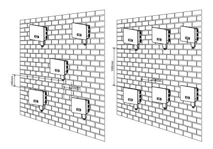
Figure 3-3 Clearance for multiple inverters
