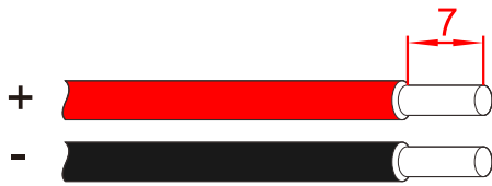
Figure3-16 Strip the PV string input wires (unit: mm)
