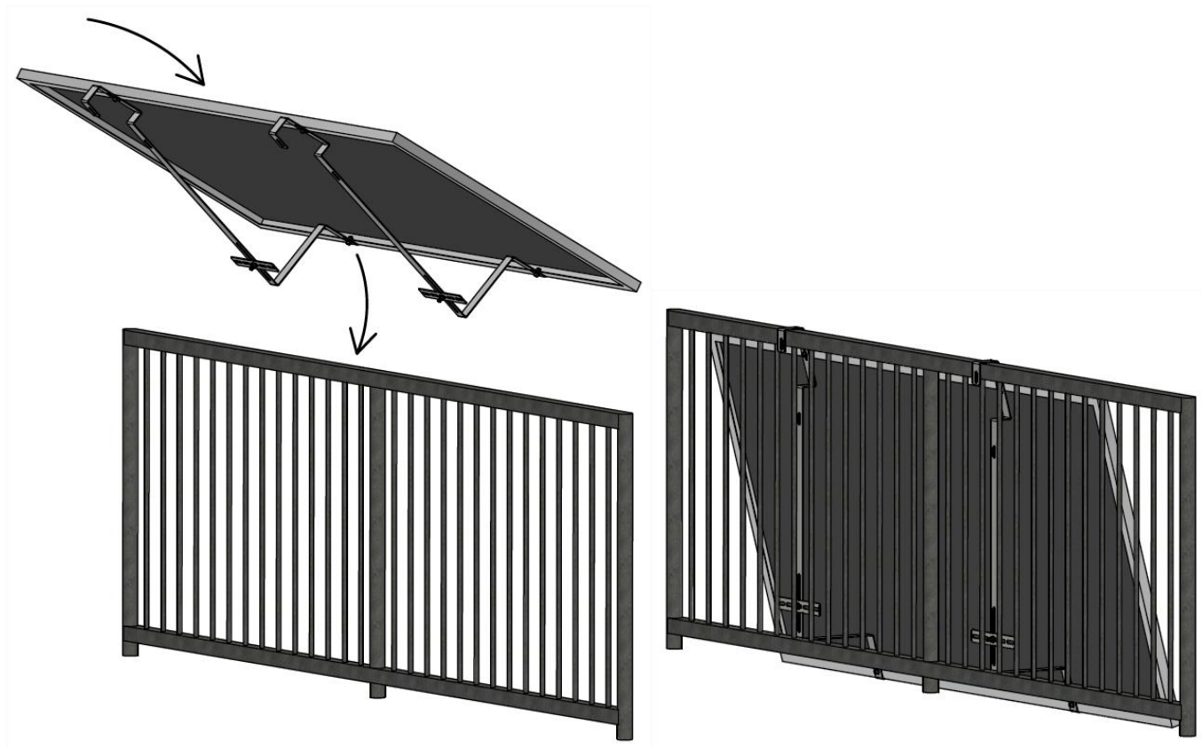
RYS.9 Installation of the structure on the railing
