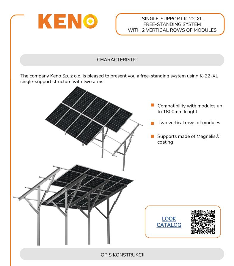
Keno Sp. z o.o. provides a 10-year warranty for the above structure with possibility of extending it by another 5 years. Supports of the structure is made with Magnelis coating, it means that the warranty for the system can be extend even up to 25 years. Structure is prepared to install 2 vertical rows of modules. Recomended maximum lenght of single table is 20 meters.
