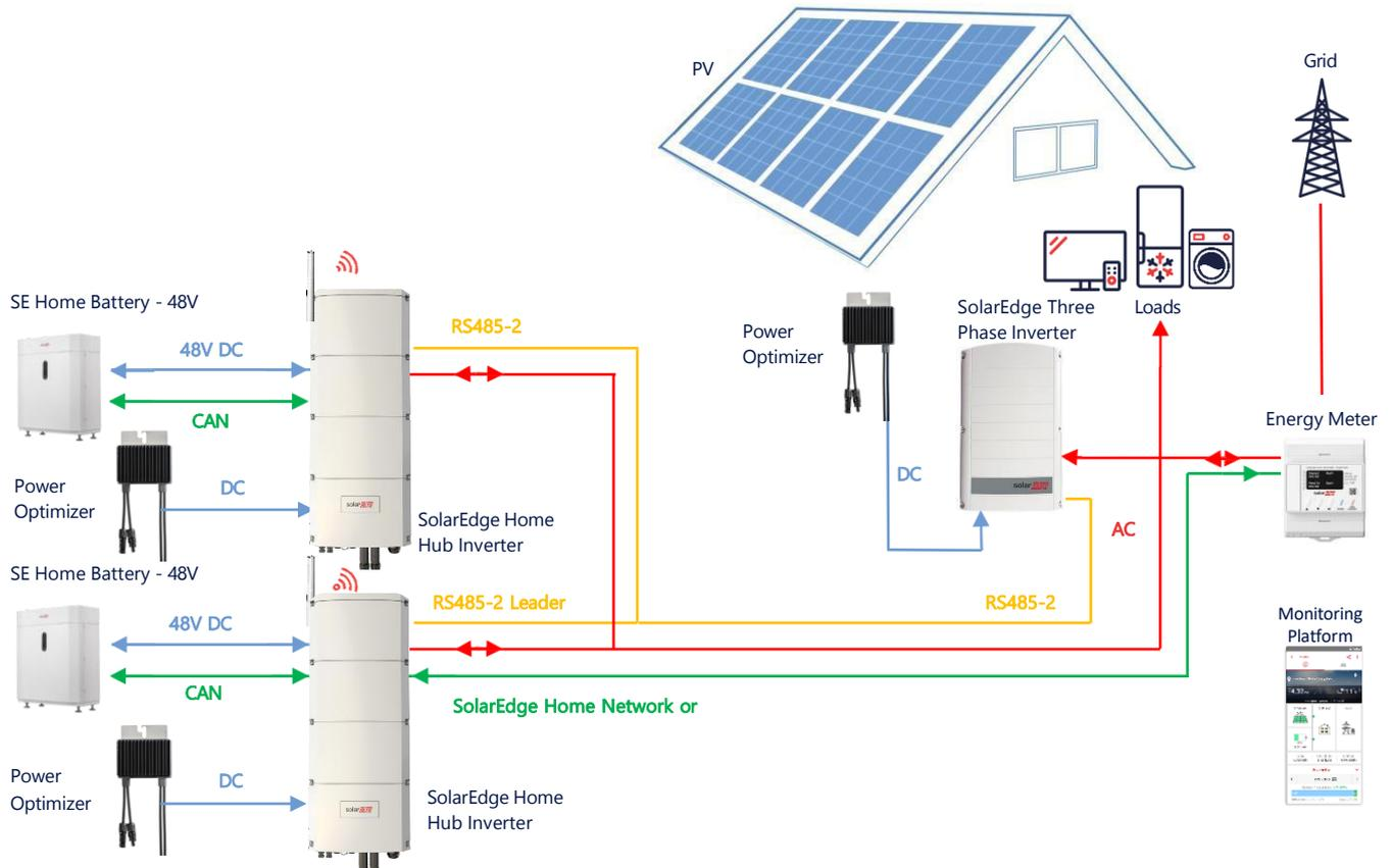
Up to three Home Hub Inverters can also have Power Optimizers or can be AC-Coupled to a non-SolarEdge power source. In case three Home Hub inverters are used with other three phase inverter from SolarEdge, the other inverter CANNOT be connected to the leader as a follower. In other words, no more than 3 inverters can be connected on a leader-follower configuration.
