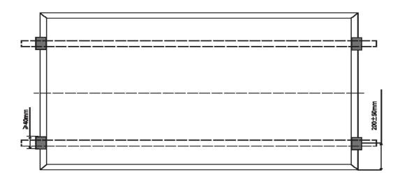
Short side clamp installation (clamp length≥40mm)
