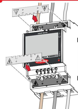
5 CONNECT THE DATA CABLES (Step: 5) → 6 SET UP THE TERMINATING RESISTOR (Steps: 6-7) → 7 → 8 MOUNT THE CONNECTOR COVERS (Step: 8) → 9 SWITCH ON THE CIRCUIT BREAKER (Step: 9)
