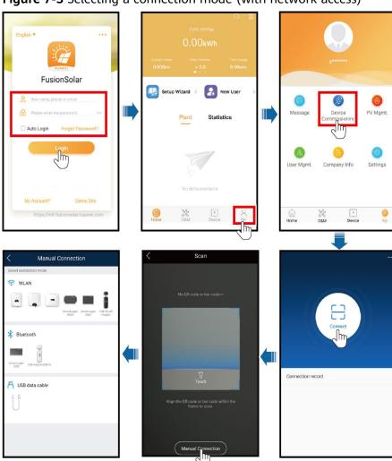
Figure 7-3 Selecting a connection mode (with network access)
