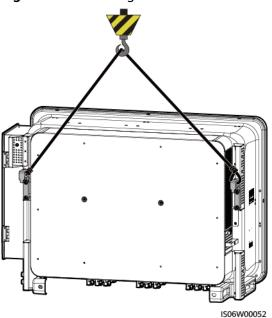
Figure 4-17 Hoisting the inverter
