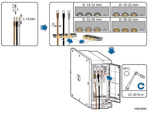
Figure 5-10 Cable connection
