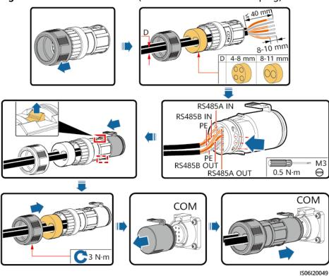
Figure 5-17 Cable connection (4-8 mm four-hole rubber plug)
