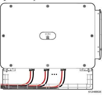
Figure A-3 Placing Y-branch connectors
