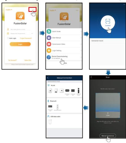
Figure 7-4 Selecting a connection mode (without network access)
