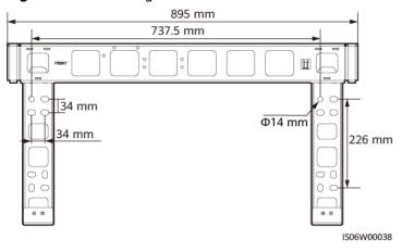
Figure 4-9 Mounting bracket dimensions
