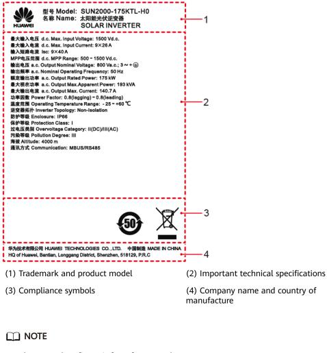
Figure 2-5 Nameplate (SUN2000-175KTL-H0 is used as an example)
