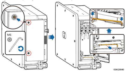
Figure 5-4 Opening the maintenance compartment door
