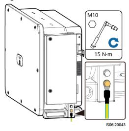
**Step 2** (Optional) Apply silica gel or paint on the ground terminal to protect it against corrosion.
