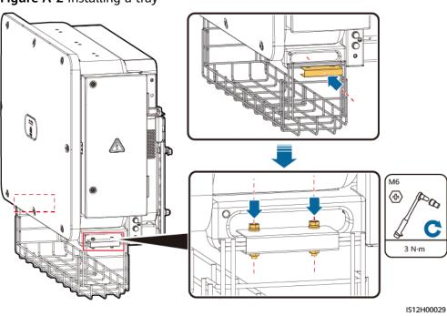
Figure A-2 Installing a tray
