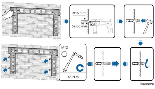
Figure 4-12 Securing the mounting bracket
