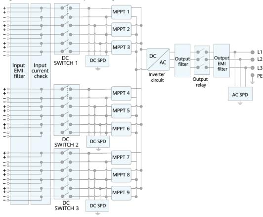
Figure 2-6 Inverter conceptual diagram
