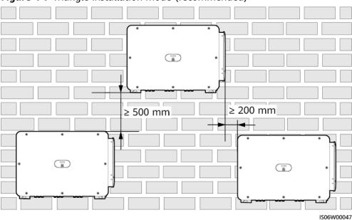
Figure 4-7 Triangle installation mode (recommended)
