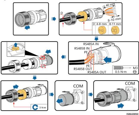
Figure 5-18 Cable connection (4-8 mm two-hole rubber plug)
