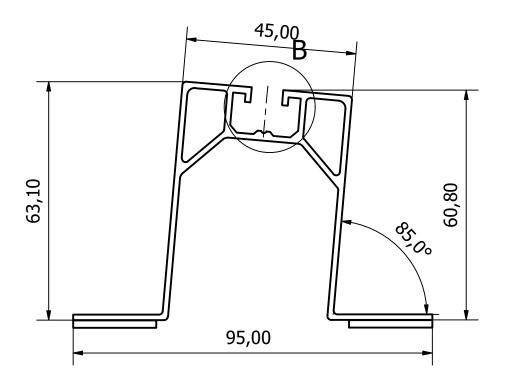
Fig. 1 Dimensions of the K-56 element
