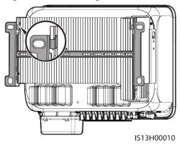
**Step 3** Tighten the nuts on both sides of the SUN2000.
