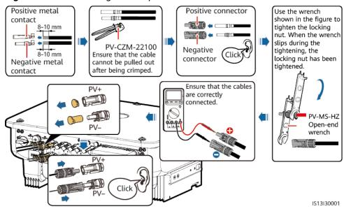
Figure 5-11 Connecting the DC power cable
