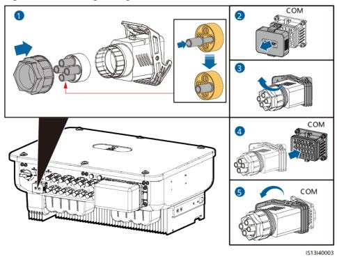
Figure 5-16 Securing the signal cable connector
