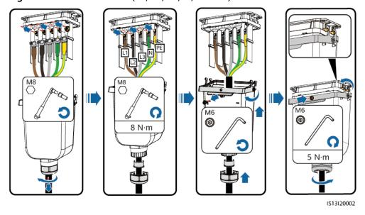
Figure 5-7 Four-core cable (L1, L2, L3, and PE)
