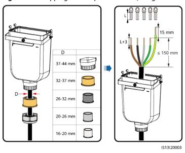
Figure 5-6 Five-core cable (L1, L2, L3, N, and PE)
