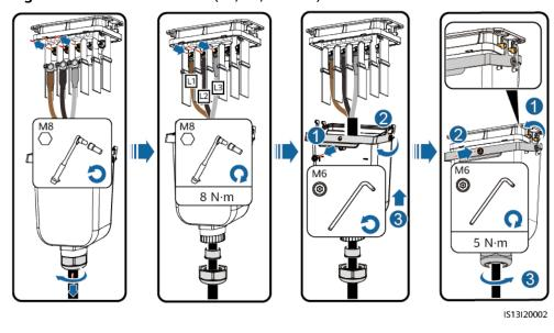
Figure 5-9 Three-core cable (L1, L2, and L3)
