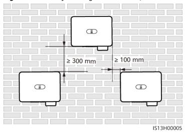
Figure 4-5 Three-layer triangle installation (not recommended)
