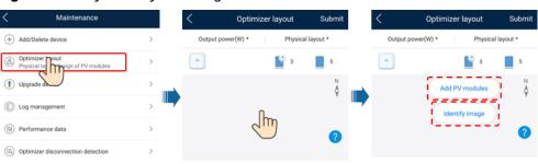
Figure 7-7 Physical layout design of PV modules
