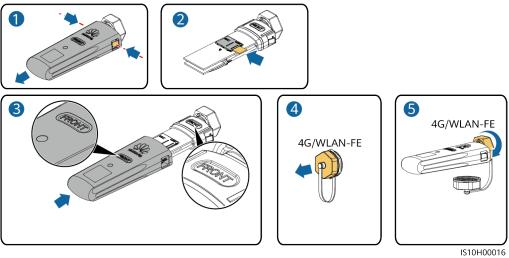
WLAN-FE Smart Dongle (WLAN Communication)
