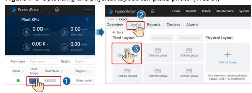
Figure 7-5 Uploading the physical layout template photo (WebUI)
