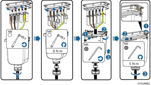
Figure 5-8 Four-core cable (L1, L2, L3, and N)
