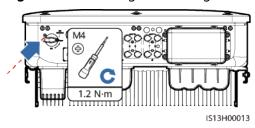
**Step 5** Turn on the DC switch between the PV string and the SUN2000 if there is any.
