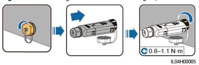
• WLAN-FE Smart Dongle (FE Communication)
