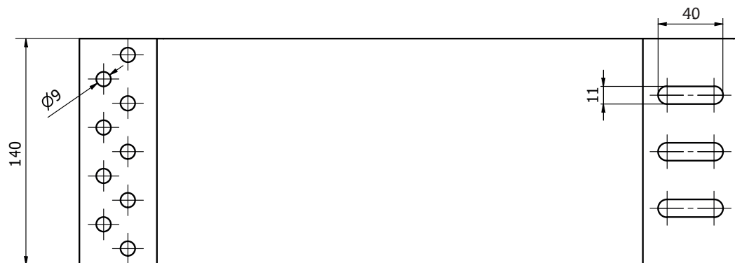
Fig. 2 Dimensions of the K-44 element - top view.
