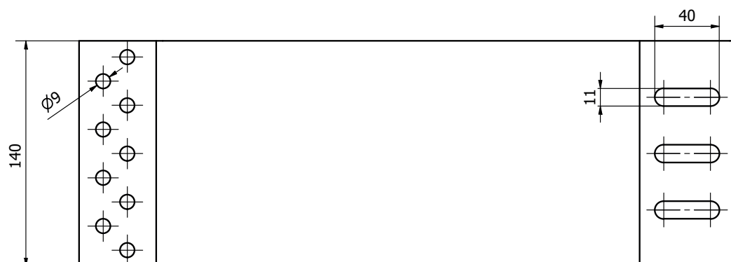
Fig. 3 Dimensions of the K-44-W element - side view
