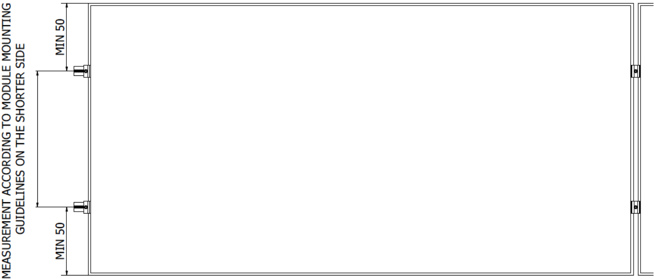
FIGURE 6 Dependence of the edge of module to the center of the module clamps
