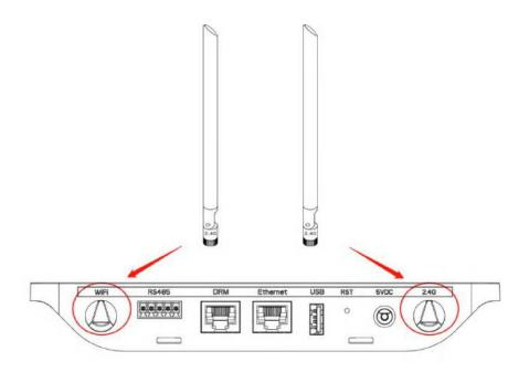
**Note :** If the DTU installation location is inside the metal box or under the metal / concrete roof, extended 2.4G cable or 2.4G sucker antenna will be suggested, which can be purchased from Hoymiles or local electrical store (Please contact Hoymiles's Tech. support team for the detail type of the cable or antenna at support@hoymiles.com).
