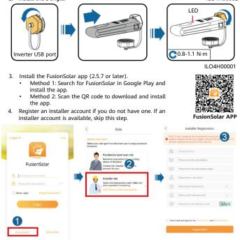
Log in to the app using the installer account, and tap Setup Wizard to create a PV plant. 5. For details, see the FusionSolar App Quick Guide.
